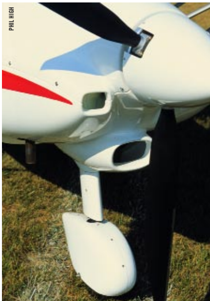
The C42 comes standard with the 80-hp Rotax 912 as its powerplant. The latest version of the aircraft added more cowling inlets to improve the flow of cooling air to the engine...a necessity in the warmer climates of the United States.
