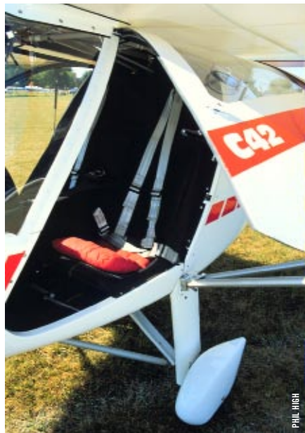
The C42's door open upward, making entry and exit easy. Gas struts hold the doors open. The aircraft can also be flown with the doors off. Inside, the aircraft features semi-bucket-style seats with a four-point shoulder harness.
