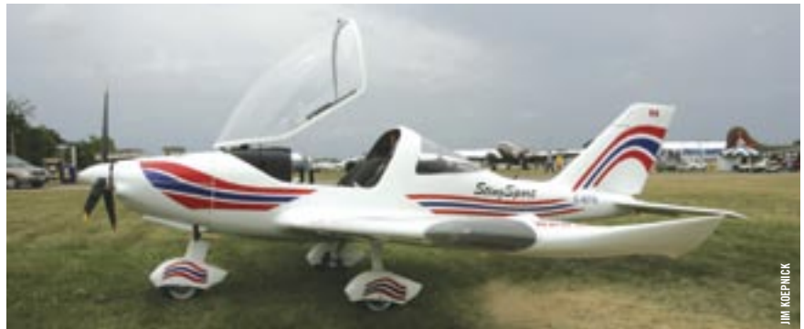
The large clear canopy pivots forward on a hinge at the front of the canopy and locks on both sides and at the rear. Dual gas struts assist in raising and lowering the canopy. Entry is gained by stepping up on the wing root and lowering oneself into the cockpit.
